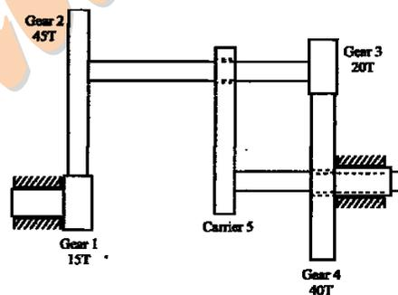
40. What is the relation between the angular velocities of Gear 1 and Gear 4?
