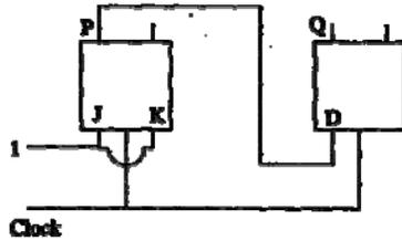
has the initial state of P, Q as 0, 1 (respectively). After three clock cycles the output state P, Q is (respectively),
