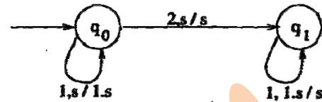
The nodes denote the states while the edges denote the moves of the pda. The edge labels are of the form  $d, s/s'$  where  $d$  is the input symbol read and  $s, s'$  are the stack contents before and after the move. For example, the edge labeled  $1, s/1.s$  denotes the move from state  $q_0$  to  $q_0$  in which the input symbol 1 is read and pushed to the stack.
